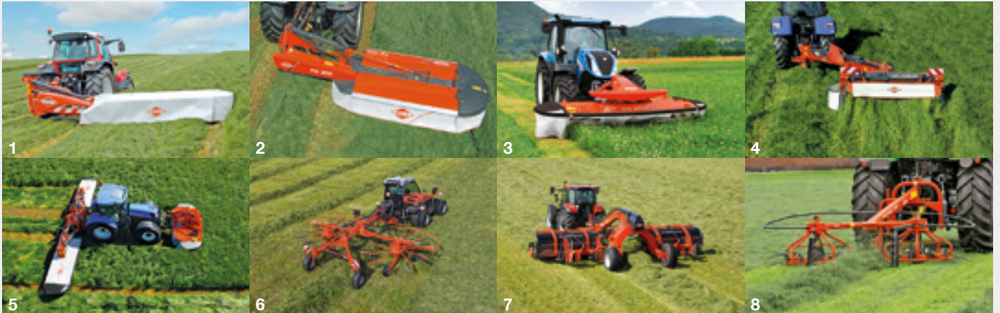
1. Rear disc mowers - 2. Rear drum mowers - 3. Front mowers and mower conditioners - 4. Rear disc mower conditioners - 5. Triple gang mower conditioners - 6. Gyrorakes - 7. Belt mergers - 8. Tedder - rakes
