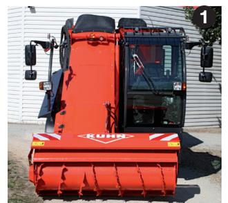
To boost the loading rate, the conveyor (2) is 800 mm wide. Therefore, the fodder flow transits quicker to the hopper. The belt is driven by a hydraulic motor at the top of the conveyor. As a result, the belt is drawn by the motor which helps to centre it.
