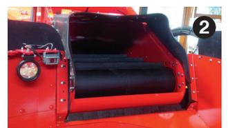
The conveyor delivers the fodder flow in the same rotational direction as the mixing augers (3). The mixing capacity does not hinder silage cutting performance!
